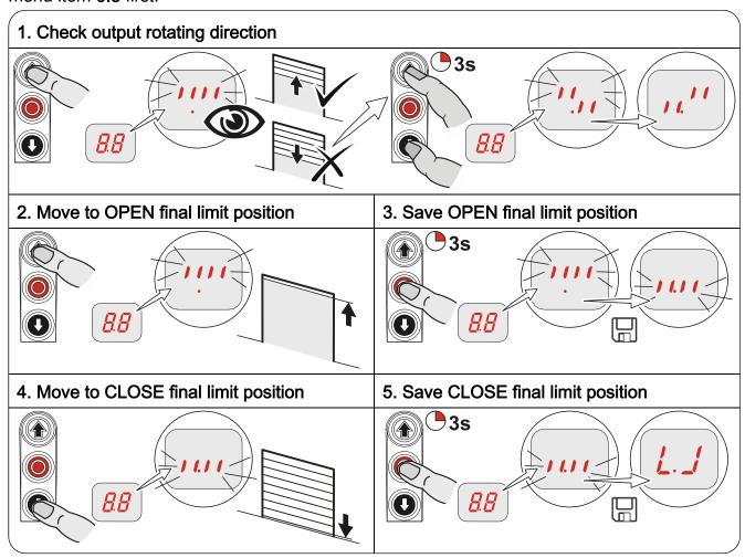
After rapid adjustment of the final limit positions, the door operating mode "hold-to-run" is active. The final limit positions can be corrected later with menu items **1.1** to **1.4**. The pre-limit is set automatically with safety edge connected. A correction is possible using menu item **1.5**.
